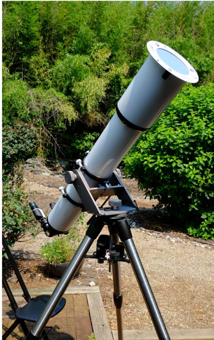
Solar observing through the 152 Apo using the ASTF exceeded all my expectations. The optical train for my observations included a Baader Zeiss T2 prism diagonal, William Optics binoviewers, and a pair of Takahashi 18mm LE eyepieces. The level of additional detail in this setup was astoundingly better compared to the 102 Apo using the standard flat glass solar filter.
