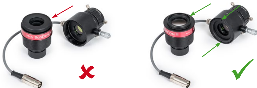
Img. 1: Unscrew the TZ-3S from the SunDancer II H-alpha-filter. Make sure that the T-2-reducer ring is inside of the H-alpha-Filter and not on the telecentric.
