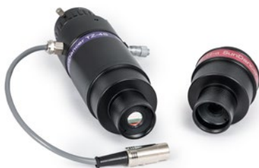
SunDancer II H-alpha-filter with TZ-4S and blocking filter, besides the original TZ-3S, now without blocking filter.
