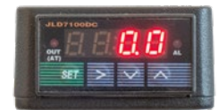
The display shows the temperature difference to the ideal operating temperature. Above shortly after powering up, below once the operating temperature is reached
