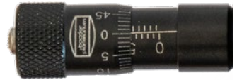
The micrometer screw can tilt the filter to easily observe the blue wing of the H-alpha-line
