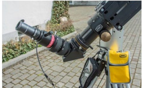
SunDancer II at a telescope with mirror star diagonal. Hand control and power supply are stored in the yellow bag.
