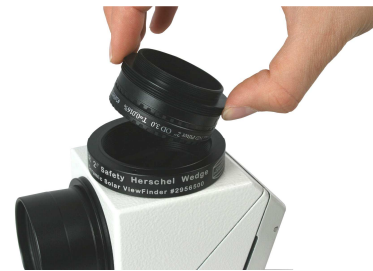
Image 6: Insert the Ring #27 with no more than two 2"-filters into the housing.
