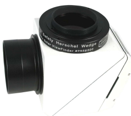
Image 7: The T2-adapter-ring is now mounted into the prism-housing.
