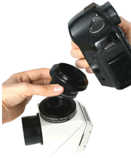
Image 10: Attach any standard T-ring (available for all standard DSLR cameras) to the T2-adapter #27
