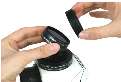
Image 4: Remove the 2"-filters from the 2" threaded ring.
