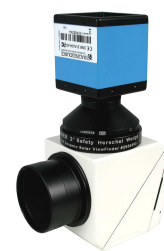
Image 9: Herschel prism with attached video module. The orientation of the camera can be changed by loosening the screws at the side of the C-Mount-adapter.
