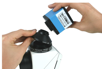
Image 8: Mounting a video module with 1" C-mount-thread onto the Herschel prism using the Baader C-Mount/T2-adapter #2958520
