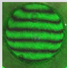
Interferogramm of a tightly locked Baader filter glass
