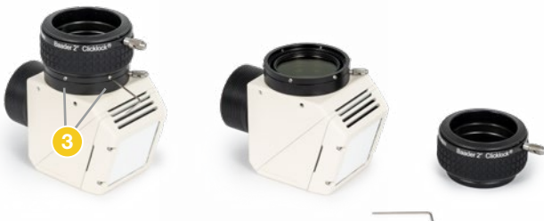
Open the six screws 3 with the 1,3 mm allen wrench, to remove the eyepiece clamp and to install e. g. a polarising filter from the top in the rotatable filter holder.
